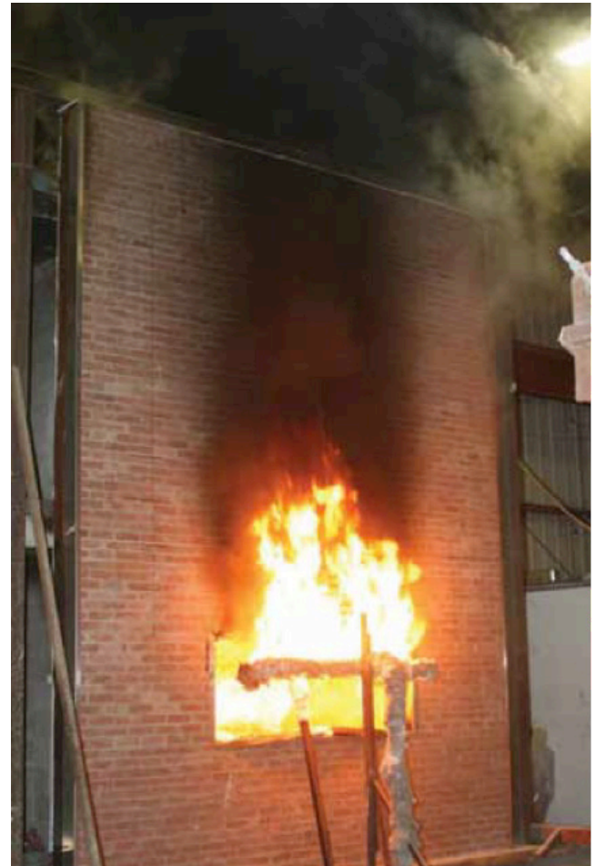
Typical example of the NFPA 285 Fire Test. Journal of Building Enclosure Design, Summer 2012, “NFPA 285: What You Need to Know”
