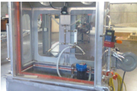
VaproShield water testing chamber calibrated to deliver 5 gal. per sq.ft. per hour, or the equivalent of 8" of rainfall per hour, with a calibrated spray rack and pressures simulating +/- 100 mph wind conditions.
