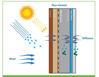
A common yet problematic solution to prevent reverse vapor drive is the installation of an exterior vapor barrier. Although installing an exterior vapor barrier will prevent the inward vapor drive, it will also stop any outward drying of the wall system through the barrier. It seals *out* vapor, but seals *in* any trapped moisture.
