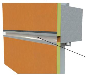
Use a combination of VaproBond sealant and VaproSilicone Transition Sheet between floors to accommodate floor line movement joints.
