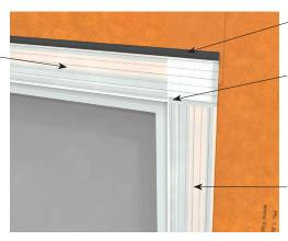
Fillet joint created by tooling VaproBond over top edge of VaproSilicone Transition
