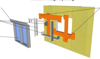
WrapFlashing SA Self-Adhered applied directly to sheathing + folded 2.75" inside of R.O.
