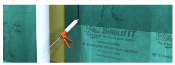
Overlap vertical seams by a min. 12". Apply  $\frac{1}{4}$ " (6.4mm) bead of VaproBond adhesive to ensure water and air barrier seal. For complete installation instructions, visit VaproShield.com
