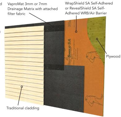
VaproMat creates a drainage cavity behind the cladding material. Install VaproMat over the WRB/AB layer with the filter fabric (black) facing outward.
