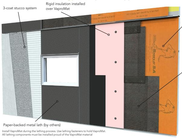
WrapShield SA Self-Adhered or RevealShield SA Self-Adhered WRB/Air Barrier
