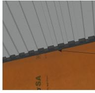
Fluted Deck Transition Install 2" (51 mm) of Vapro-Liqui-Flash onto metal deck and 2" (51 mm) onto wall
