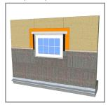
15. Install metal head flashing with end dams, (by others).
