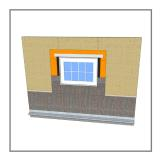
12. Fold drainage mesh back onto wall trimming around window frame. Tack mesh in place with stapler or hammertacker.
