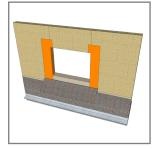
6. Install WrapFlashing SA at jambs as shown. Cut at sill and head and fold into rough opening.
