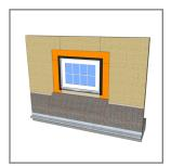
11. After window installation, seal nail flanges at jambs and head with VaproLiqui-Flash or VaproTape.
