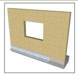
1. Install WrapFlashing SA course at base of wall to foundation. Install metal flashing by others.
