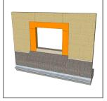
7. Install WrapFlashing SA at head as shown. Cut at jambs and fold into rough opening.
