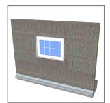
17. Install next horizontal course of RSSA over headflashing. Notch and trim if required to fit.
