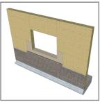
5. Carefully detach mesh and fold down 2" below sill. Cut WRB/AB material flush with jambs and fold into sill.
