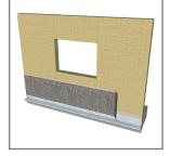
2. Install first course of RSSA field material overlapping base flashing by 2" min.
