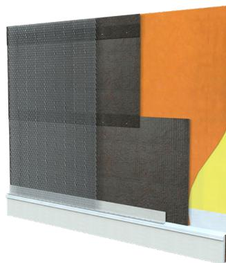
8. Install expanded metal lath over the VaproMat according to the manufacturers' recommendations. Consult NW Wall and Ceiling Bureau, [nwcb.org](http://nwcb.org), for details regarding drainage stucco systems. All lath including weep screeds are installed "proud" or over the VaproMat material.
