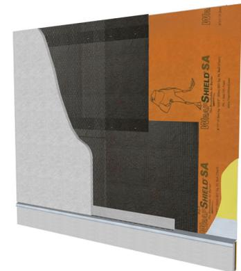
9. Apply stucco according to manufacturers' recommendations. Guidelines should include a weep method for ventilation and drainage as recommended by Northwest Wall and Ceiling Bureau details [www.nwcb.org](http://www.nwcb.org).
