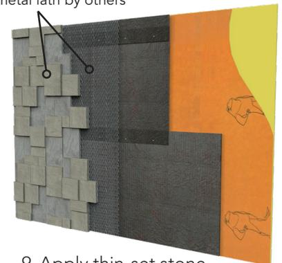
9. Apply thin-set stone according to manufacturers' recommendations. Guidelines should include a weep method for ventilation and drainage as recommended.
