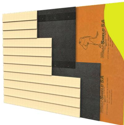
8. Install wood siding, shingles and fiber-cement siding according to manufacturers' recommendations.
