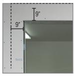
2. Measure and cut WrapFlashing SA sill, left & right jambs, and head flashing so that each piece extends 9" past edges of opening for each side (= R.O. + 18").
