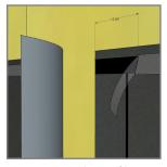
5. Remove release film from top of tape where flap overlaps.
