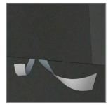
7. Join horizontal seams by peeling back both release films, starting from where horizontal joint meets vertical joint.
