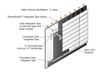
Apply a single layer of **RevealShield IT Integrated Tape** Water Resistive Vapor Permeable Air Barrier Membrane to create the desired black open joint.
