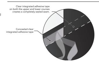
Clear Integrated Tape protected by the 6" horizontal lap allows easy installation in all weather conditions.
