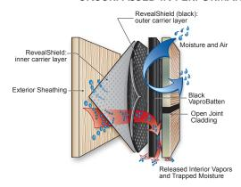
RevealShield IT Integrated Tape, UV stable membrane for open joint cladding, membrane construction.
