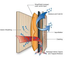
WrapShield IT WRB/Air Barrier is vapor open, allowing trapped moisture to escape and air tight preventing costly air migration.
