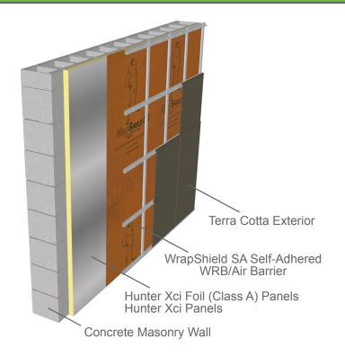
Comprehensive details available at VaproShield.com. **Materials Wall Component** Illustration for explanatory purposes only. **Base Wall System**
