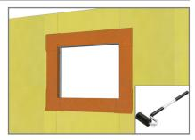
3. Install head piece with 2.75" folded into R.O. 9" to be left on face. Roll all WrapFlashing SA (orange) sections with weighted roller to ensure full contact.
