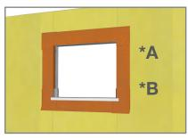
4. Install Vapro-SS Flashing at sill in shingle fashion with 3" up-turned legs at sill and head + 1" on face; jambs are 1" onto the face.
