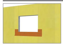
1. Install WrapFlashing SA Self-Adhered into sill with 2.75" folded into Rough Opening (R.O.) 9" left on face, with bottom 6" of release film to remain attached.
