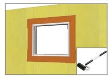
6. Install Vapro-SS Flashing on head in shingle fashion with 3" up-turned legs at sill and head + 1" on face; jambs are 1" onto the face. Roll all Vapro-SS Flashing with weighted roller to ensure full contact.
