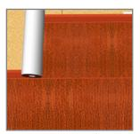
11. Secure material to substrate using only recommended gasketed fasteners in the field area of Wrap-Shield RS, as previously noted in this document. Continue up the wall in shingle fashion. Repeat as needed.
