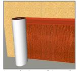
2. At the base of the wall, begin installation with SS staples in the top 2" above the tape. Snap a line for guidance. **Do not staple in the tape area.**
