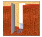
5. Remove release film of WrapFlashing SA Self-Adhered. Note: mechanically attached WrapFlashing SA may be used in lieu of WrapFlashing SA, with a 3/8" bead of VaproBond Adhesive Sealant, blind sealing behind each flap.
