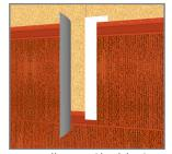
6. Install WrapShield RS abutting piece with joint centered on WrapFlashing SA. Use hand pressure to engage the pressure sensitive adhesive.
