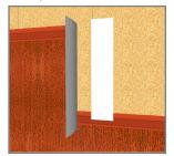
4. Staple 11 3/4" Wrap-Flashing SA Self-Adhered, centered behind vertical joint location, with white adhesive side out. Lap over lower course, halfway onto tape joint [approx. 3.5"], as shown. Place butted joint at middle of WrapFlashing SA Self-Adhered.
