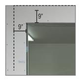
2. Measure and cut WrapFlashing SA sill, left & right jambs, and head flashing so that each piece extends 9" past edges of opening for each side (= R.O. + 18").
