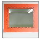
10. Using the sausage gun or DRY joint knife, apply VaproLiqui-Flash in a zigzag pattern on the wall face surrounding the rough opening.
