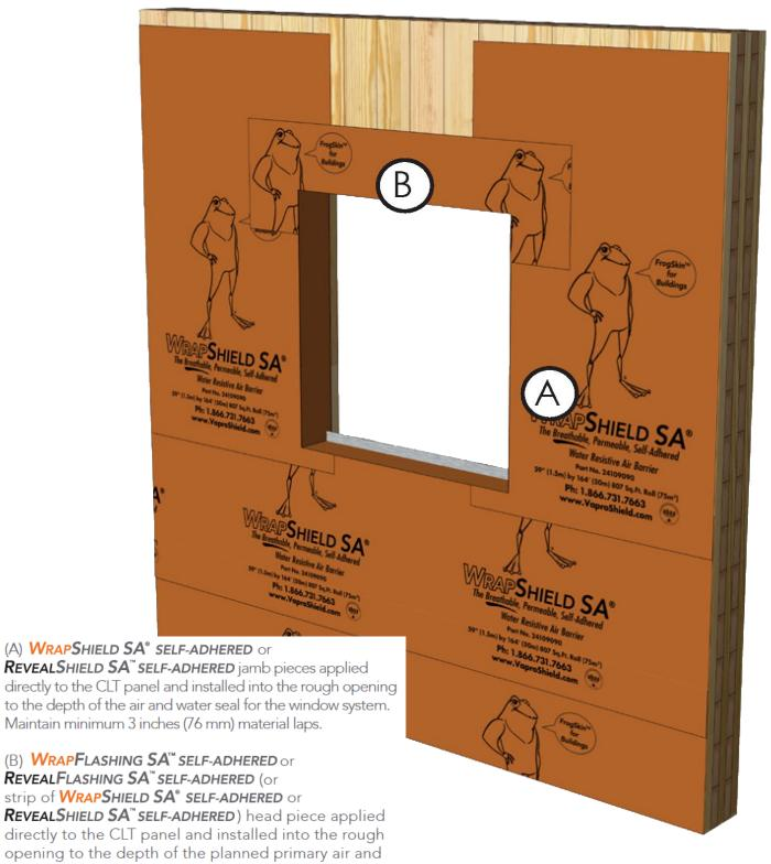
directly to the CLT panel and installed into the rough opening to the depth of the air and water seal for the window system. Maintain minimum 3 inches (76 mm) material laps. (B) WRAPFLASHING SA™ SELF-ADHERED or REVEALFLASHING SA™ SELF-ADHERED (or strip of WRAPSHIELD SA® SELF-ADHERED or
