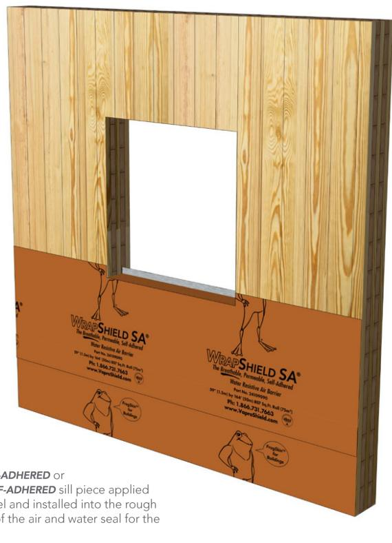
WRAPSHIELD SA® SELF-ADHERED or **REVEALSHIELD SA™ SELF-ADHERED** sill piece applied directly to the CLT panel and installed into the rough opening to the depth of the air and water seal for the window system.
