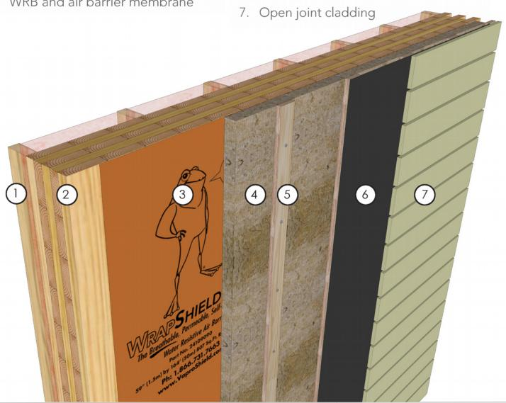
CLT with Open Joint Cladding System
