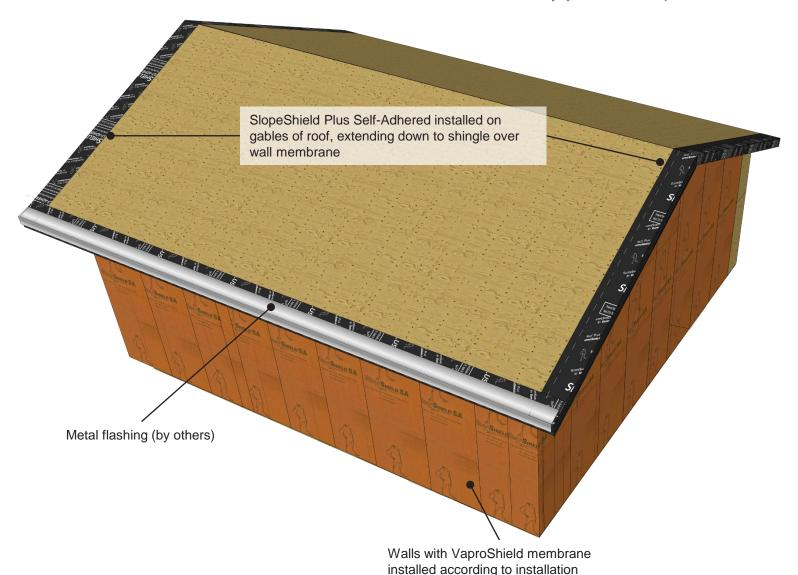
Step 4: Install metal flashing (by others) over SlopeFlashing at eaves
