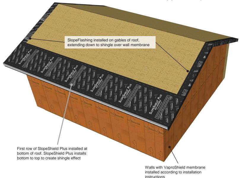
Step 5: Install first row of SlopeShield Plus Self-Adhered
