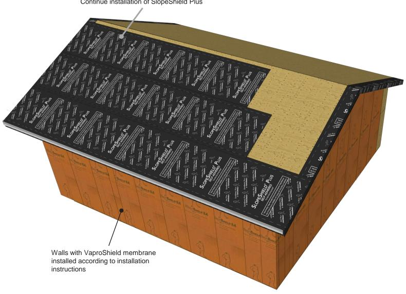
Step 6: Install up roof, maintaining 3" minimum overlap between runs of roofing material
