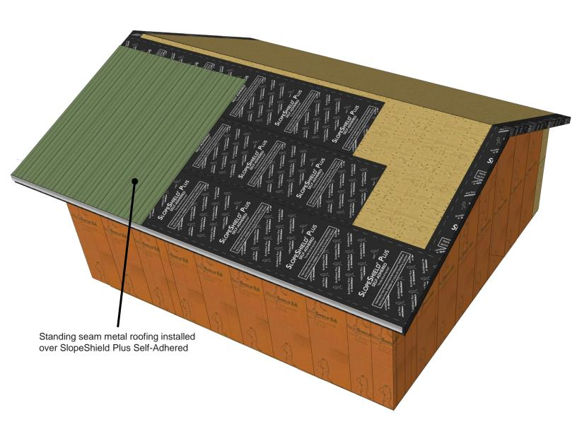
Step 7: Install Standing seam metal roofing
