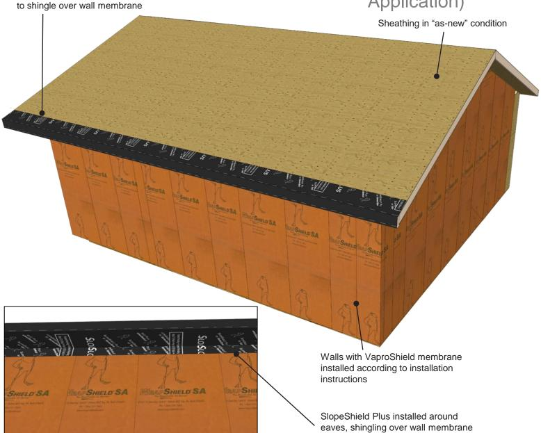
Step 2: Install SlopeFlashing around eaves, shingling over wall membrane
