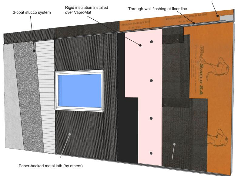
VaproMat 3mm or 7mm Drainage Matrix with attached filter fabric
