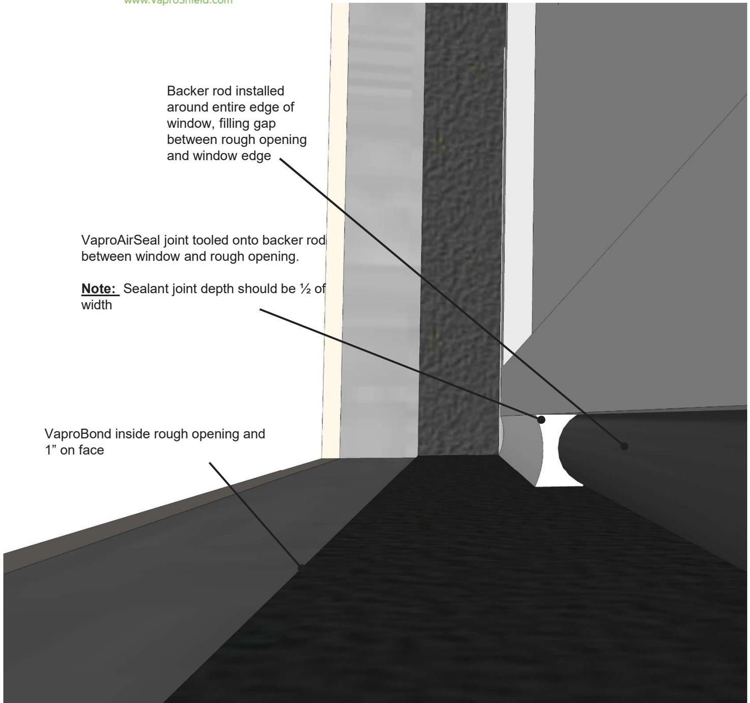
Backer rod installed around entire edge of window, filling gap between rough opening and window edge
