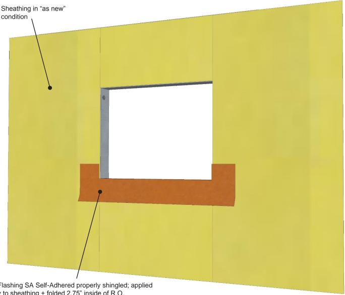
VaproFlashing SA Self-Adhered properly shingled; applied directly to sheathing + folded 2.75" inside of R.O.
