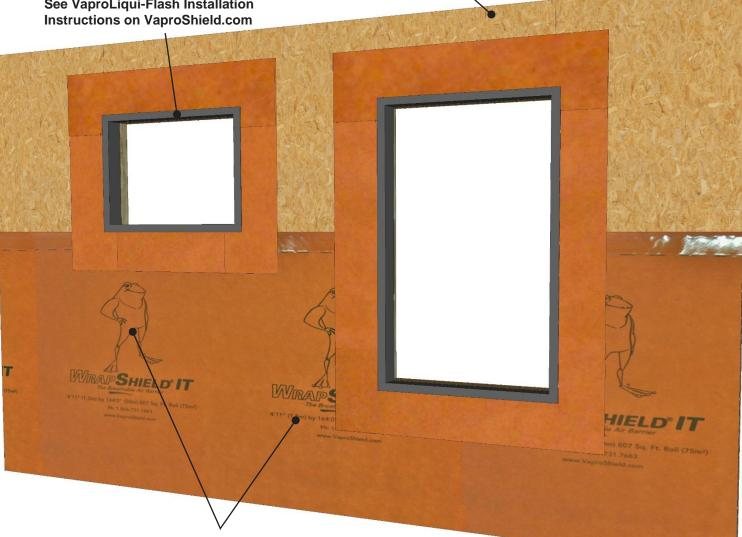
WrapShield IT Integrated Tape installed horizontally
