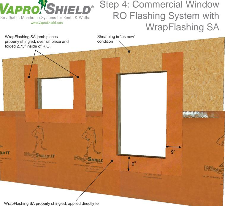
WrapFlashing SA properly shingled; applied directly to field membrane + folded 2.75" inside of R.O.
