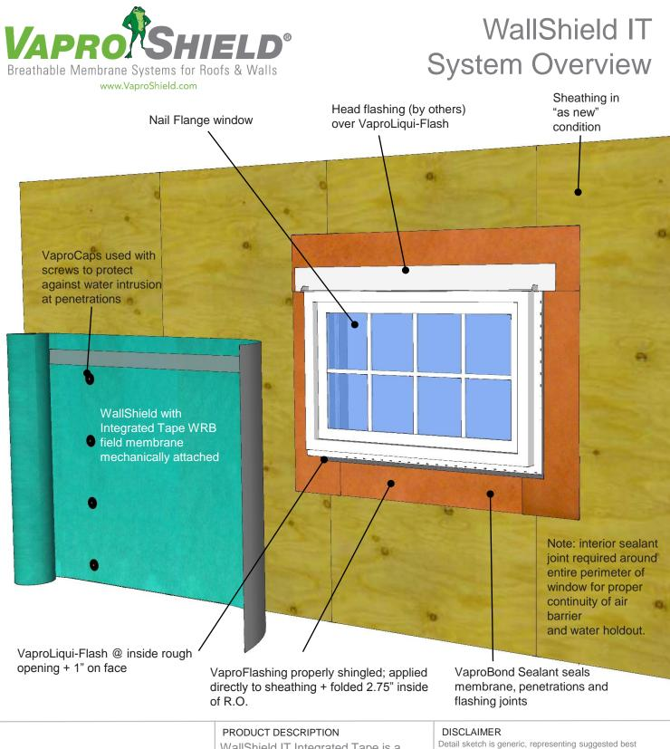
WallShield IT Integrated Tape is a primary, water resistive, vapor permeable, air permeable, mechanically attached sheet membrane for rain screen building enclosures.
