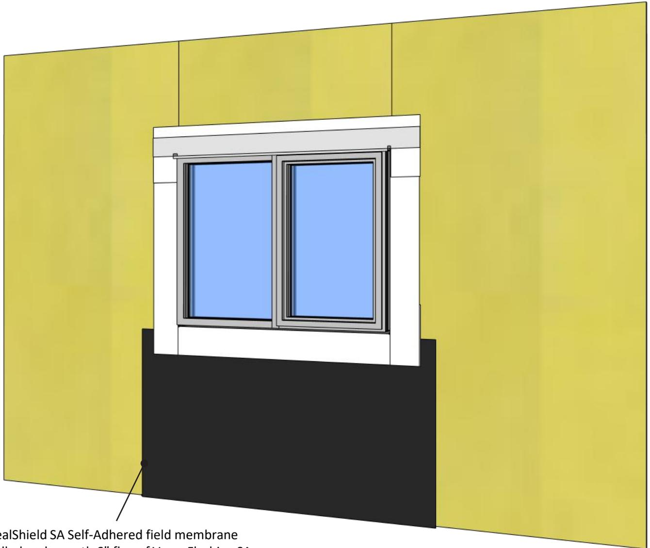
RevealShield SA Self-Adhered field membrane installed underneath 6" flap of VaproFlashing SA to create shingle effect
