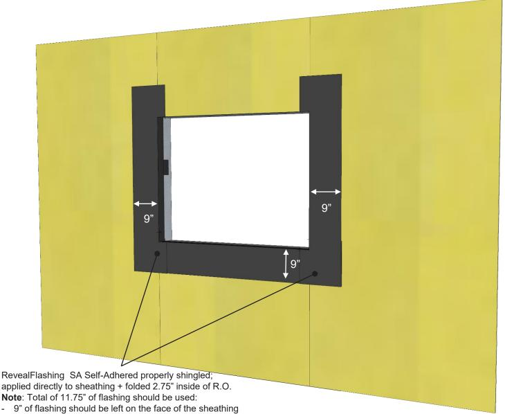
6" of release film from the bottom of the flashing to be left attached for shingling over membrane.
