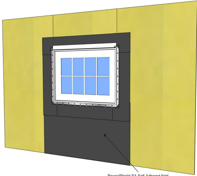
RevealShield SA Self-Adhered field membrane installed underneath 6" flap of RevealFlashing SA to create shingle effect
