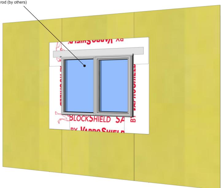
Step 4: Install commercial window w/ perimeter sealant joint and backer rod (by others). Install metal head flashing (by others) over cured VaproBond
