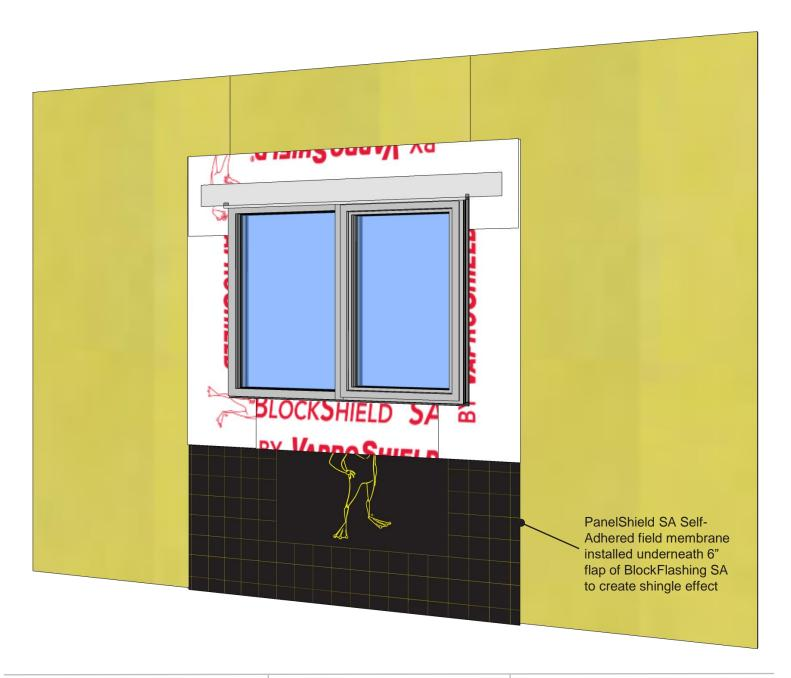
Step 5: Install field membrane, shingled underneath window flashing
