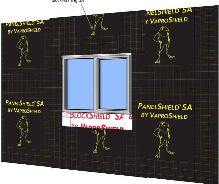
Step 7: Install field membrane over metal head flashing, maintaining 3" minimum overlap to adjacent field membrane.
