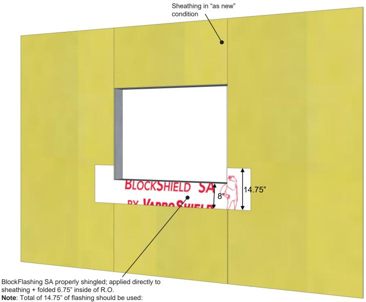
8" of flashing should be left on the face of the sheathing
