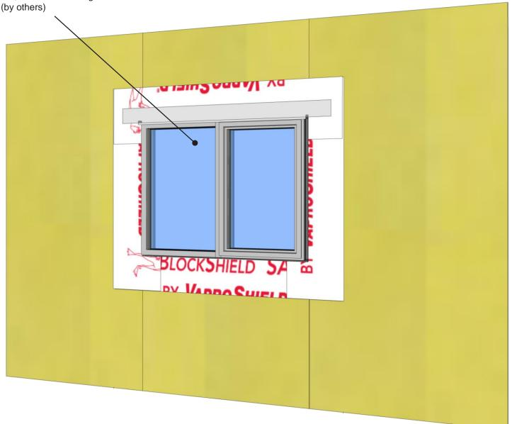
Step 4: Install commercial window w/ perimeter sealant joint and backer rod (by others). Install metal head flashing (by others) over cured VaproBond
