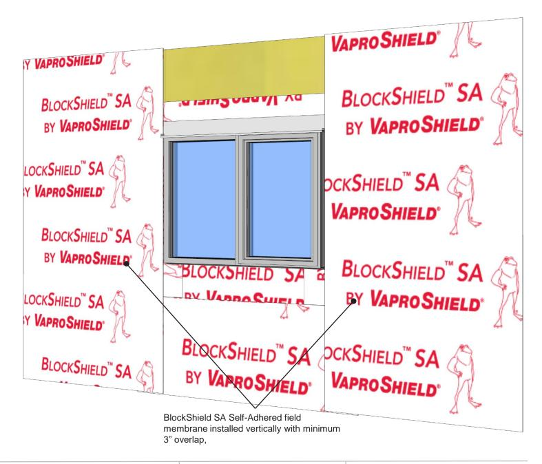
Step 6: Install field membrane vertically to sheathing, maintaining 3" minimum overlap with R.O. flashing
