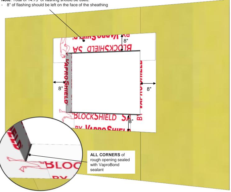
Step 3: Install head piece with 6.75" folded into R.O. 8" to be left on face.
