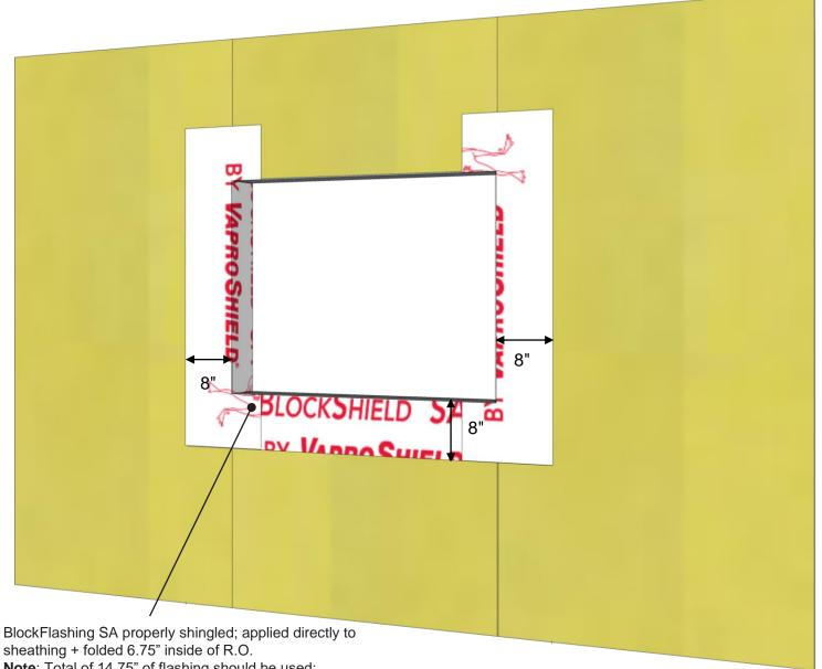
Note: Total of 14.75" of flashing should be used:
