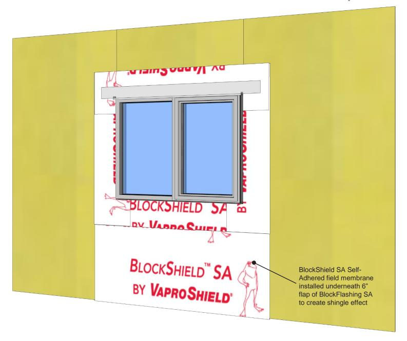
Step 5: Install field membrane, shingled underneath window flashing
