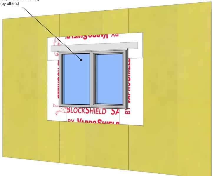
**BlockFlashing SA is designed for** locations where vapor permeability is not required. Steel framing with Densglass sheathing shown above.
