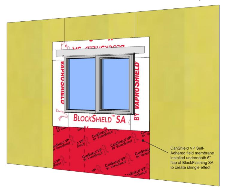
BlockFlashing SA is designed for locations where vapor permeability is not required. Steel framing with Densglass sheathing shown above.
