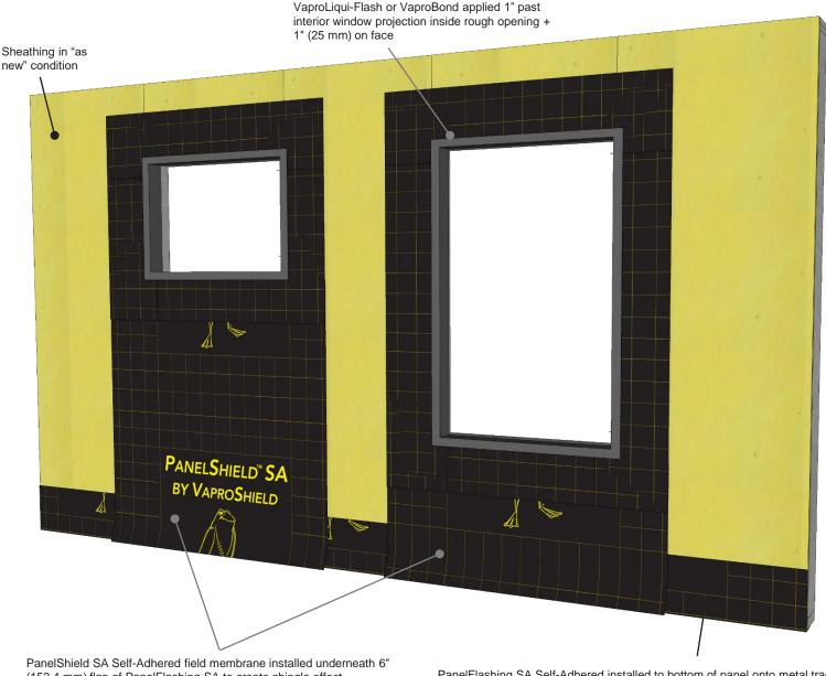
(152.4 mm) flap of PanelFlashing SA to create shingle effect
