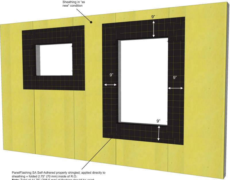
Note: Total of 11.75" (298.5 mm) of flashing should be used:
