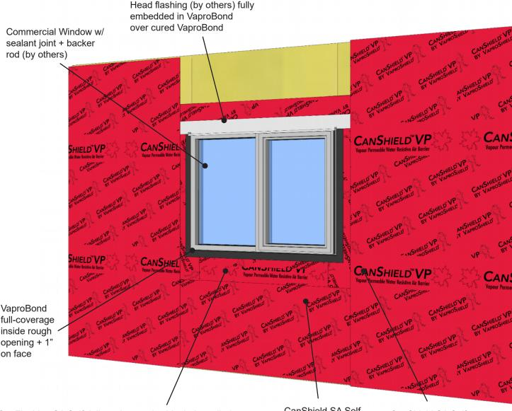
CanFlashing SA Self-Adhered properly shingled; applied directly to sheathing + folded 2.75" inside of R.O. **Note**: Total of 11.75" of flashing should be used:
