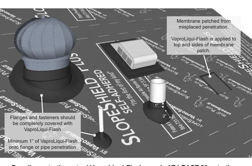
For all penetrations: tool VaproLiqui-Flash evenly AT LEAST 2" onto the face and AT LEAST 1" out along all sides of the penetration
