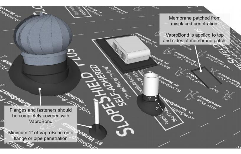
For all penetrations: tool VaproBond evenly AT LEAST 2" onto the face and AT LEAST 1" out along all sides of the penetration
