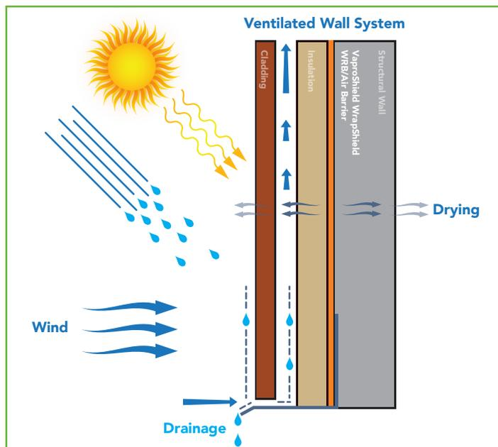
VaproShield's *Installation Best Practices* requires a rain screen or ventilated cladding design that 'vents off' the resulting vapor pressures when present. This practice prevents reverse vapor drive and allows effective drying in both directions of the wall system.
