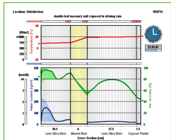
Typically, a water resistant barrier/air barrier is used to control vapor diffusion caused by reverse vapor drive. The amount of vapor restriction or transmittance is calculated using hygrothermal modeling data.
