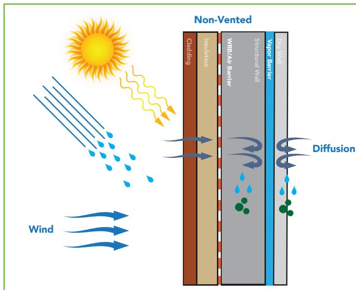
A common yet problematic solution to prevent reverse vapor drive is the installation of an exterior vapor barrier. Although installing an exterior vapor barrier will prevent the inward vapor drive, it will also stop any outward drying of the wall system through the barrier. It seals *out* vapor, but seals *in* any trapped moisture.
