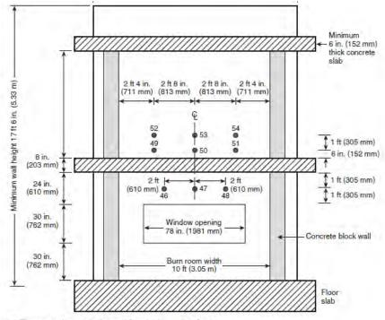
Thermocouples - 1 in. (25 mm) from interior wall surface
