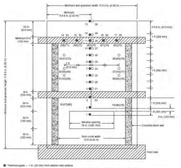
O Thermocouples - in the wait cavity air space or the insulation, or both, as shown in Figure 6.1(b) Details A through I.
