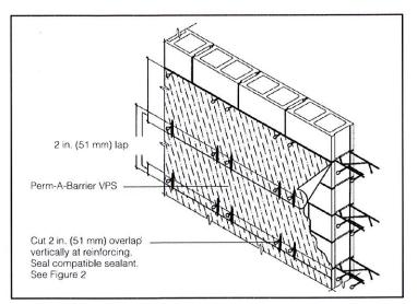
Figure 1: Membrane System Detail
