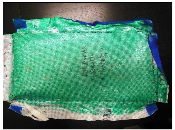
Henry VP160 with Aquatac Primer after transfer from release sheet. Post test photo.
