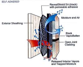
RevealShield SA Self-Adhered, UV stable membrane for open joint cladding construction.
