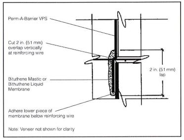
Figure 2: Horizontal Reinforcing
