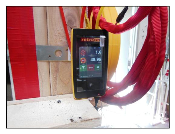
The air exchange rate of 50 ACH was chosen as it represents the likely flows associated with a properly vented  $\frac{1}{2}$ " rainscreen cavity, based on previous publications <sup>4,5</sup>, accounting for thermal and moisture buoyancy, convection due to thermal gradients, vent occlusion, and wind driven air pressure.
