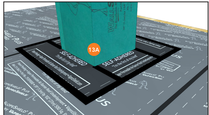
13A. Install WallShield IT over post protection to optimize mass timber protection.
