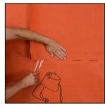
10. Use the opposite hand to smooth the two layers together as the release film is removed.
