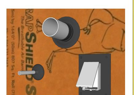
**VaproBond** is used to seal typical building penetrations. Tool at least 2" onto face and 1" along all sides of the penetration.
