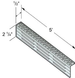
VaproVent Hook Strips are used with VaproBattens as a starter strip for vinyl and beveled siding applications, in place of the VaproVent L Strip at the bottom of the assembly.
