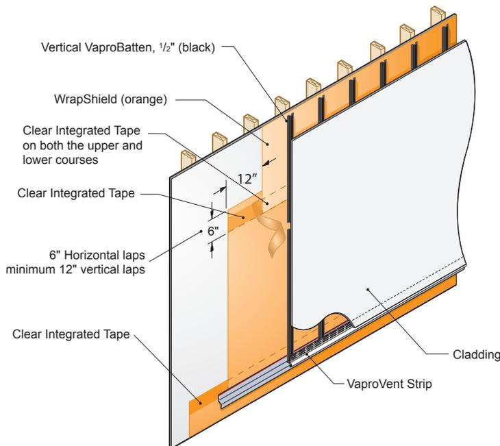
*Promote lifelong building health with VaproShield's fully tested building envelope solutions. Our system of breathable water resistive barrier membranes, battens and flashing products reduce contractor liability and excessive energy consumption for the life of the building.*
