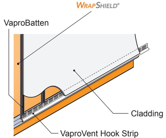
*Close-up: WrapShield using Rain Screen Design Components: VaproBatten and VaproVent Hook Strip*
