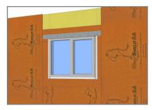
8. Install field membrane vertically to sheathing, maintaining 3" minimum overlap with R.O. flashing, roll to ensure adhesion at seams (overlaps).
