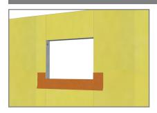
1. Install WrapFlashing SA Self-Adhered into sill with 2.75" folded into Rough Opening (R.O.) 9" left on face, with bottom 6" of release film to remain attached.
