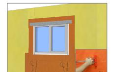
7. Install field membrane underneath 6" flap of sill flashing to create shingle effect, remove release film, adhere to membrane, roll to ensure adhesion at seams (overlaps).
