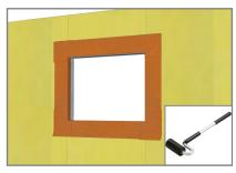
3. Install head piece with 2.75" folded into R.O. 9" to be left on face. Roll all WrapFlashing SA (orange) sections with weighted roller to ensure full contact.
