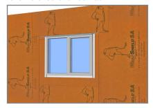
9. Install WrapShield SA field membrane over metal head flashing, maintaining 3" minimum overlap to adjacent field membrane. roll to ensure adhesion at seams (overlaps).
