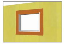
5. Install Vapro-SS Flashing at jambs in shingle fashion with 3" up-turned legs at sill and head + 1" on face; jambs are 1" onto the face.
