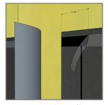
5. Remove release film from top of tape where flap overlaps.
