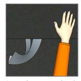
9. Use the opposite hand to smooth the two layers together as the release film is removed.
