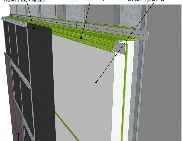
Open Joint Rain screen cladding material (by others)
