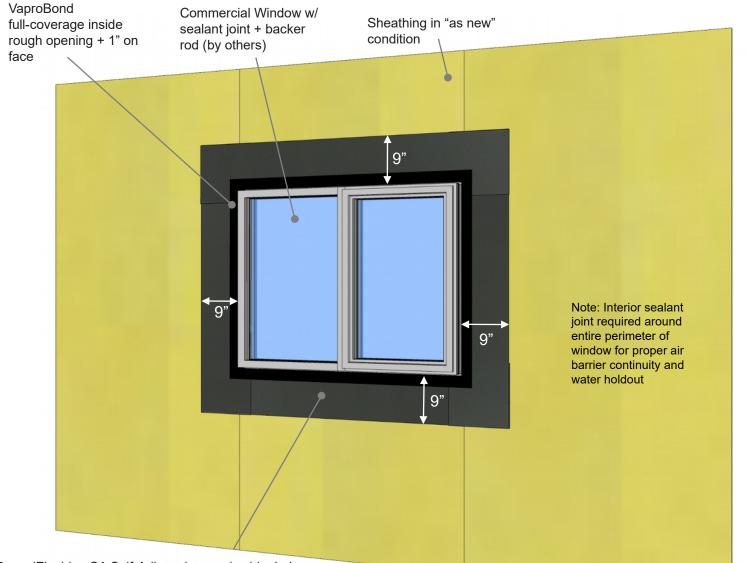
RevealFlashing SA Self-Adhered properly shingled; applied directly to sheathing + folded 2.75" inside of R.O. **Note**: Total of 11.75" of flashing should be used:
