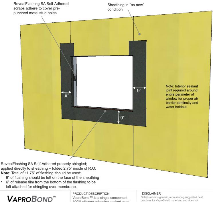
Step 3: Install jamb pieces with 2.75" folded into R.O. 9" to be left on face.
