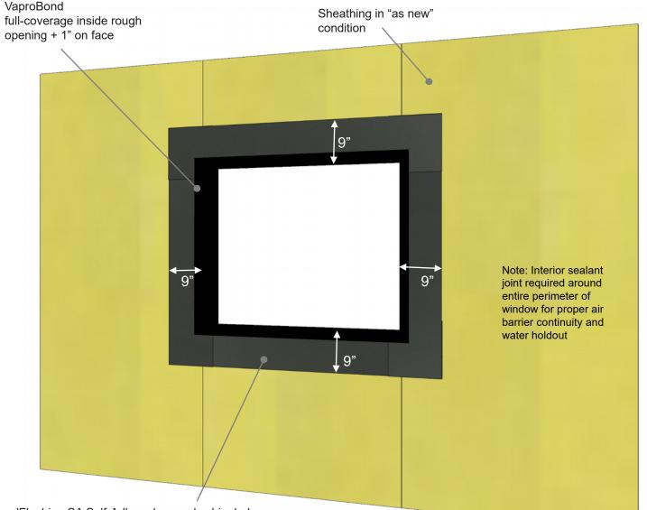
RevealFlashing SA Self-Adhered properly shingled; applied directly to sheathing + folded 2.75" inside of R.O. Note: Total of 11.75" of flashing should be used:
