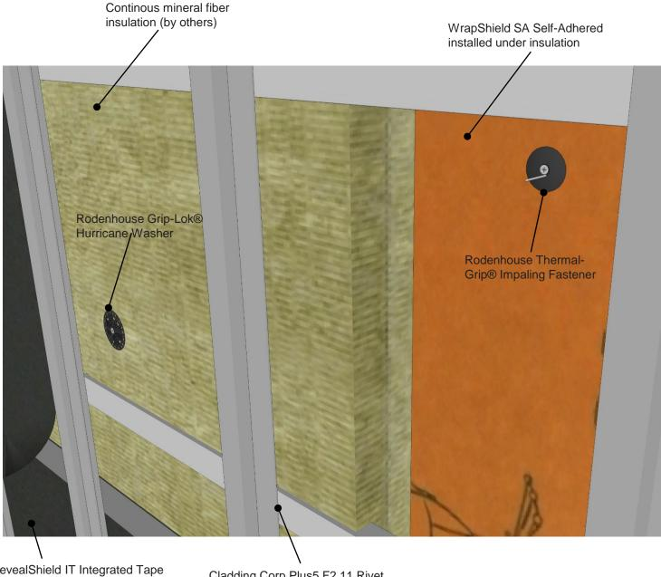
RevealShield IT Integrated Tape installed over mineral fiber insulation and horizontal girts
