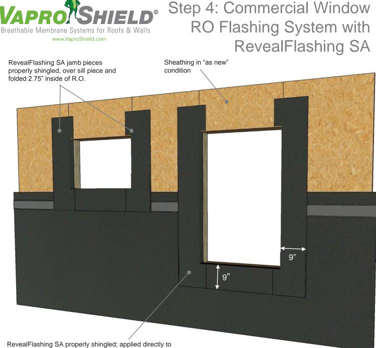
RevealFlashing SA properly shingled; applied directly to field membrane + folded 2.75" inside of R.O.
