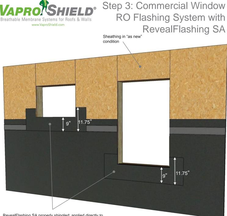
RevealFlashing SA properly shingled; applied directly to field membrane + folded 2.75" inside of R.O. **Note**: Total of 11.75" of flashing should be used:
