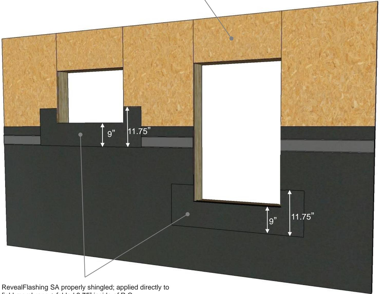
RevealFlashing SA properly shingled; applied directly to field membrane + folded 2.75" inside of R.O.
