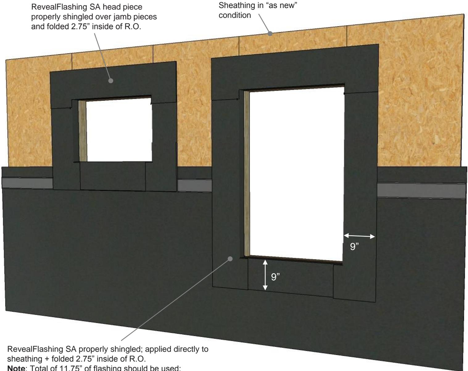
RevealFlashing SA properly shingled; applied directly to sheathing + folded 2.75" inside of R.O.
