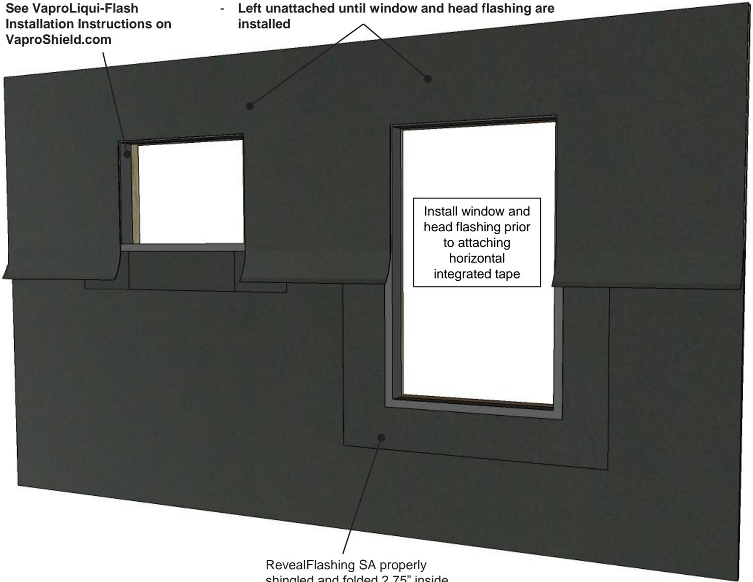
RevealFlashing SA properly shingled and folded 2.75" inside of R.O.
